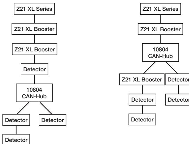
If there is no CAN socket on the control panel, the **Z21 XL BOOSTER** can alternatively be connected to the Z21 Series control panel via a four-pole B-Bus cable socket using a four-pole B-Bus cable (10757) to the Z21 Series control unit via the "B-Bus socket". With older control units, the connection may also be designated as "booster out". In this case it is irrelevant which of the two sockets is used on the booster.
