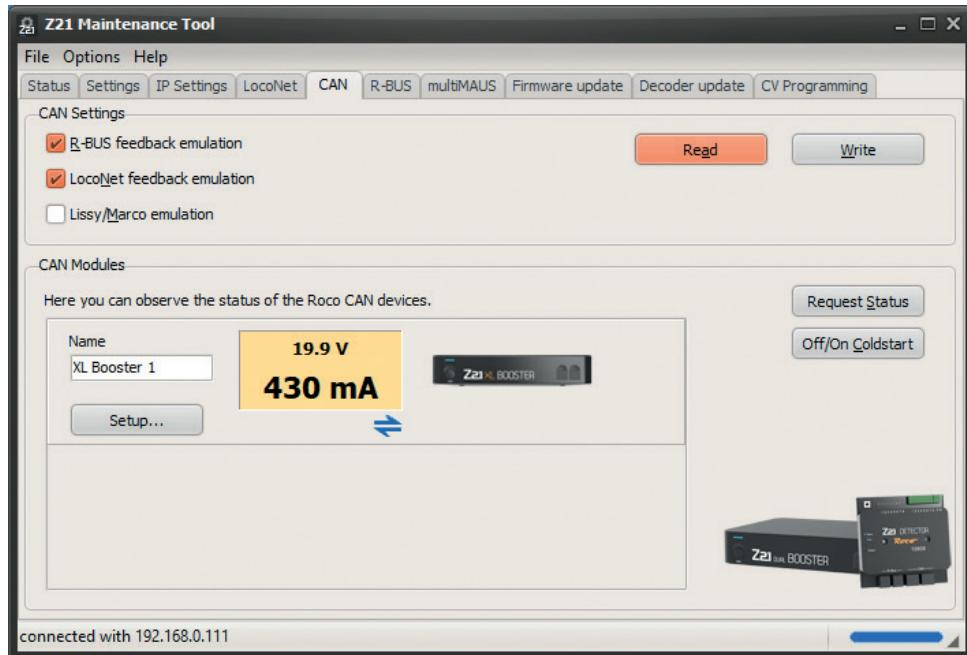
A panel appears for each Z21 Booster output with the current voltage and current consumption of the respective track output. By clicking on the field, you can conveniently activate or deactivate the corresponding booster output from the PC for the aim of troubleshooting (booster management).
