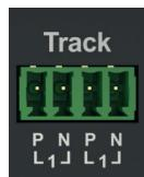
The **Z21 XL BOOSTER** has two equivalent, internally connected track connections that can deliver a total of a maximum of 6 A.
