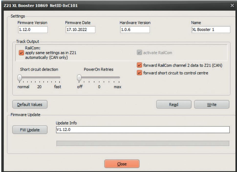
**RailCom:** Automatically accept settings from the central unit via CAN (= "Auto Settings", activated by default).
