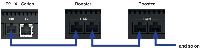
The Z21 XL BOOSTER is preferably connected to the Z21 XL Series control panel via the CAN cable supplied. It is irrelevant which of the two CAN sockets is used at the booster. The CAN bus not only
