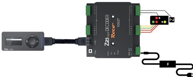
Alternatively, the Z21 pro LINK can also be supplied via a USB power port. In this way, the Z21 pro LINK can also supply the connected zLink-compatible device. To do this, use the 10859 - USB 5 Watt switching power supply.
