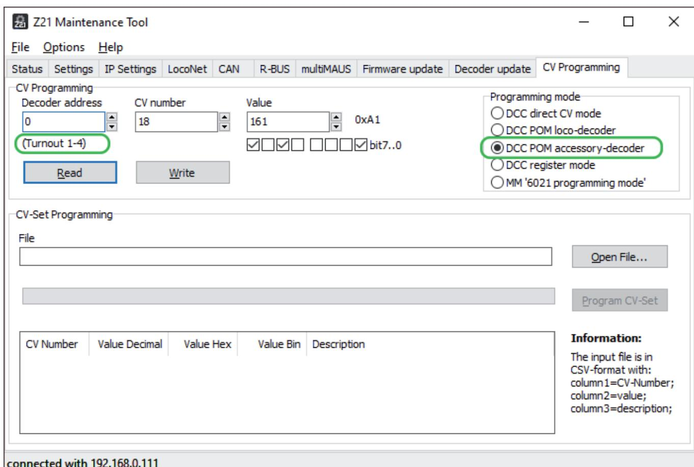
It is essential to ensure here that the correct turnout address/decoder address has been selected before reading or writing so that the desired switch decoder is also actually actuated with the programming commands.
