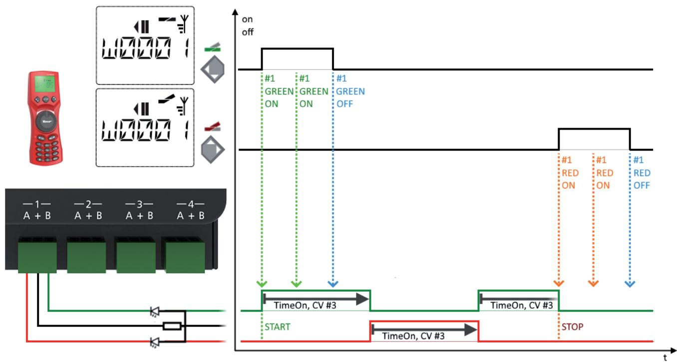
Optionally also available with slow fade-up and fade-down (light bulb simulation).
