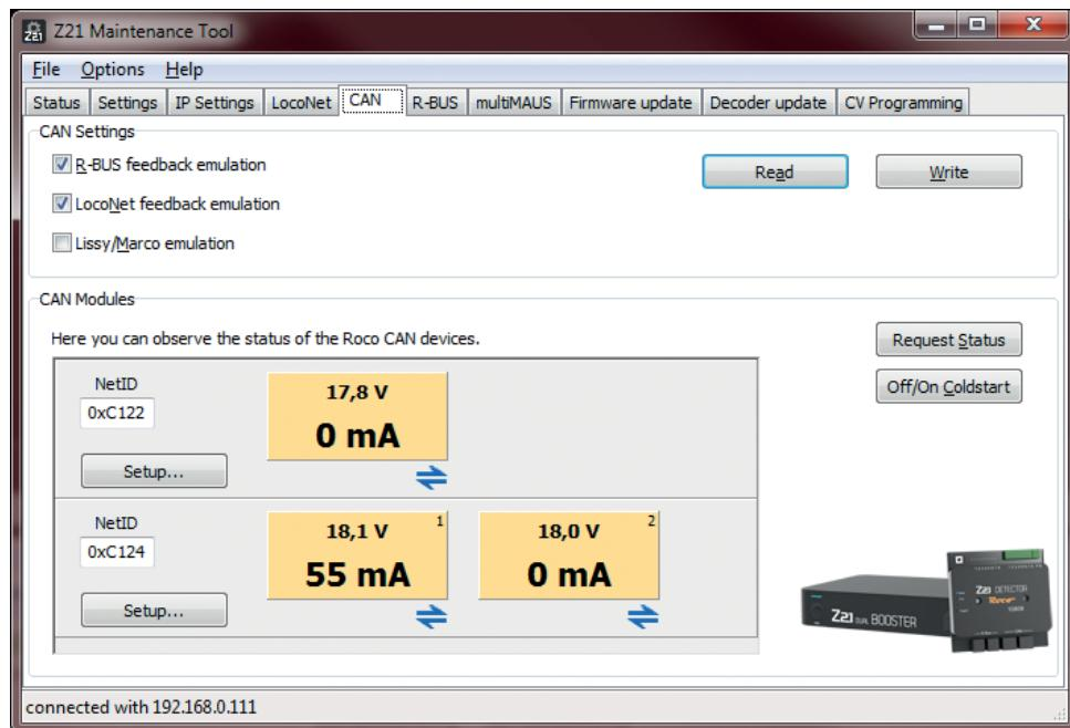
One or two panels showing the single or dual booster, depending on the type together with the current voltage and the current consumption for the corresponding track output.
