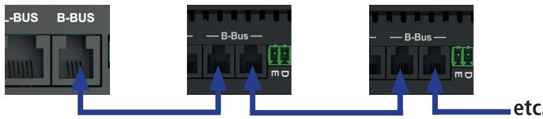
The Z21-Boosters can also be connected to the Z21 or the Z21start by inserting the enclosed four-pin B-Bus cable in the "B-Bus" socket. It is possible that this connection is designated as "Booster out" on older control centres. Which of the two sockets is used is unimportant.
