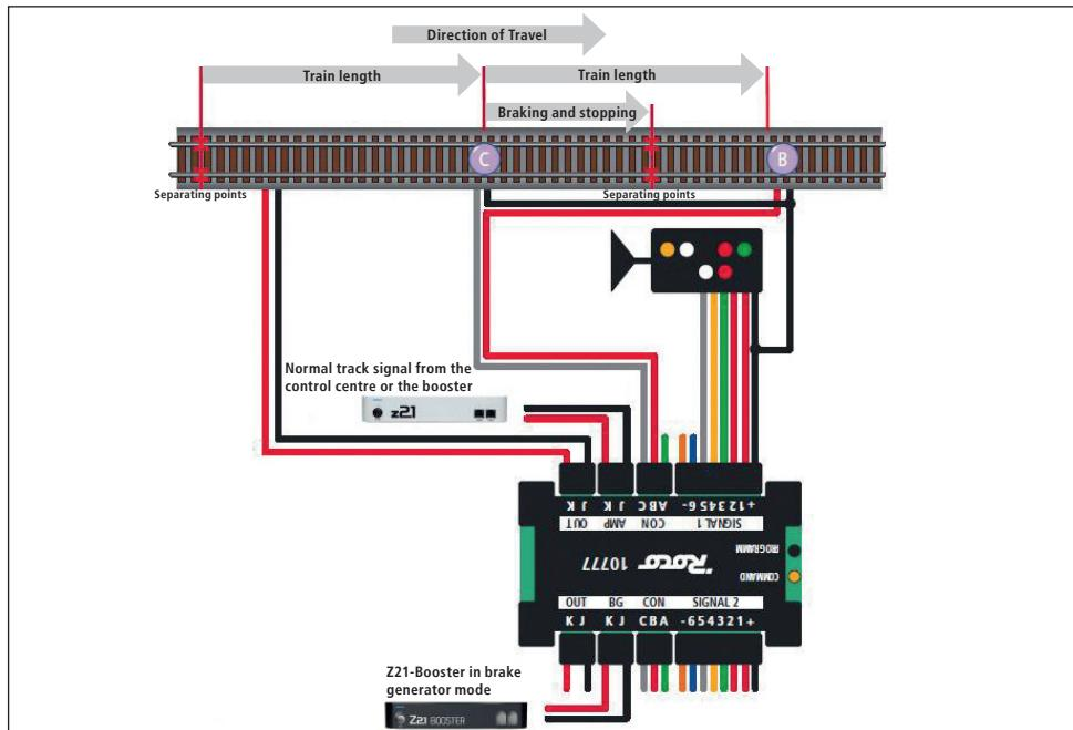
The length of the stopping section corresponds with a maximum train length plus the braking distance (alter the decoder setting if necessary).
