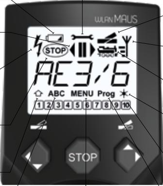
**Battery symbol** shows the charge status of the batteries
