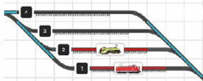
Detail from the Z21 schematic signal box of the Z21 app - when using the Z21 DETECTOR (10808) in addition to the feedback message a picture of the locomotive is shown.
