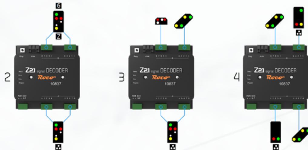
Depending on the complexity of the different signals, a varying number of devices can be connected.
